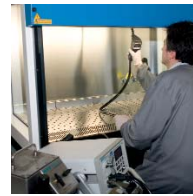
FILTER LEAKAGE TEST
