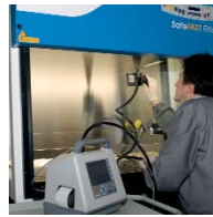
FILTER LEAKAGE TEST
